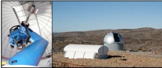
JAST/T80 Telescope: 83cm diameter, 2deg Field of View (left)
