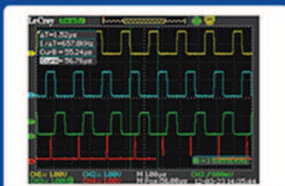
Fig.3 - The read phases of CCD (R1s) with a configurable Clamp signal. It can clamp the output value in the optimal instant of charge.
