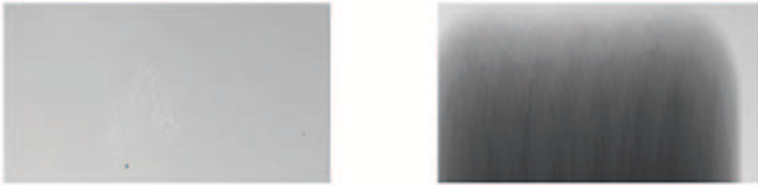
Fig.1 - The image shows a reading of a CCD with a good CTE (left) compared to one that has been degraded (right)
